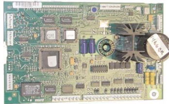
Merlin 4 Control Board
