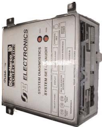
Dixie SII Control Box
